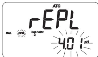
Use the arrow keys to select the buffer to be replaced, then press CFM to confirm or CAL to exit calibration without replacing.
