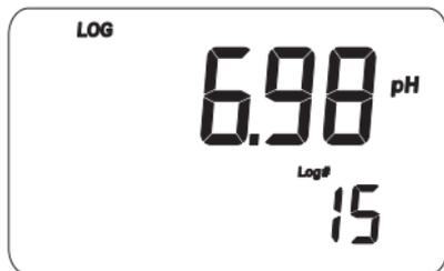
Pressing SHIFT and then SETUP key while in memory recall mode, the secondary LCD will toggle between the lot and the record number. Use the arrow keys to select a different lot or record.
