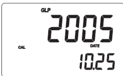
Use the up arrow key to view all calibration parameters in the following sequence:
