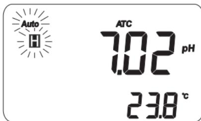
When the reading is stable, the “Auto” and “H” tags stop blinking and the reading is frozen.
