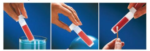
The addition of environmentally friendly biodiesel to the fossil diesel offers microbes an excellent source of nutrition. Microbes grow more than ever and form increased amounts of "biomass". This leads to clogged filters, corrosion and to engine failure.
